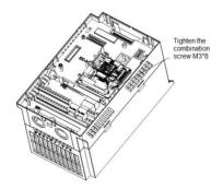
Figure 4 CANopen Expansion Card Installation
