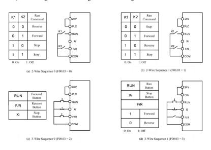
Figure 1-6 Control Logic of Terminal Control Mode
