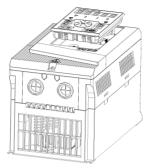
Figure 2-4 Keypad Installation
