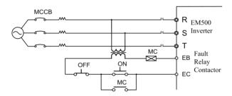
Figure 3-5 Connecting to Input Circuit Breaker
