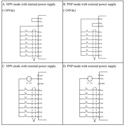
Figure 3-17 Wiring of Multi-function Input Terminals
