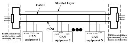
Figure 13-1 CAN bus topology diagram
