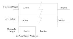
Figure 7-14 Numeric Output Terminal Level and Monopulse Output
