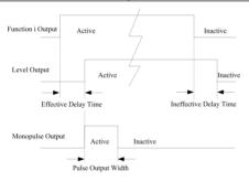
Figure 7-16 Numeric Output Terminal Level and Monopulse Output
