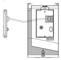
Figure 3-25 Wiring of Keypad Extension Line
