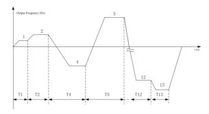
Figure 7-26 Simple PLC Running
