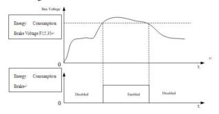
Figure 7-39 Energy consumption brake
