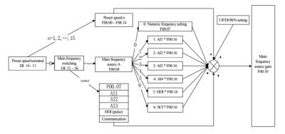
Figure 1-2 Main Frequency Source A Setting
