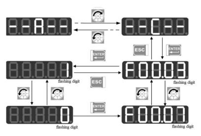
Figure 4-7 Changing Function Parameters under Non-Factory Defaults Mode
