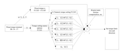
Figure 1-5 Torque Setting Mode
