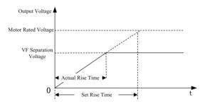
Figure 7-21 Voltage Rise Time of VF Separation
