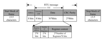
Figure 12-1 RTU Message Frame
