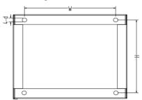
Figure 11-4 Installation Dimensions of Anchor Bolt of Base
