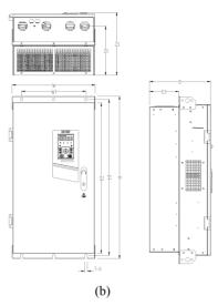
Figure 2-8 Installation Dimensions for Flush Mounting
