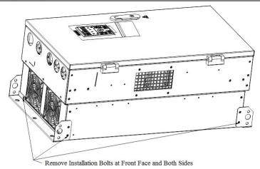
Figure 2-5 Disassemble Top and Bottom Mounting Holes
