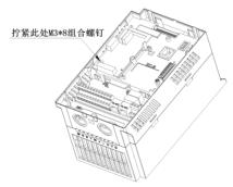
Figure 6 IO expansion card installation diagram
