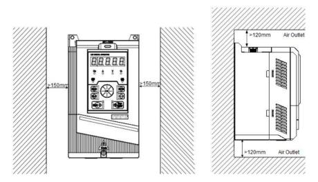
Figure 2-2 Inverter Installation Direction and Space
