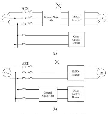
Figure 3-7 Incorrect Installation of Noise Filter
