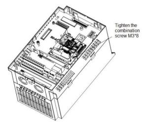
Figure 5 Installation of DeviceNet Expansion Card
