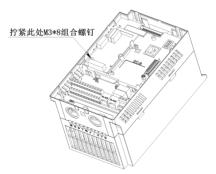
$Figure\ 5\ IO\ expansion\ card\ installation\ diagram$
