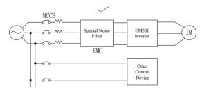
Figure 3-6 Correct Installation of Noise Filter
