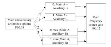
Figure 1-4 Main and Auxiliary Arithmetic Setting
