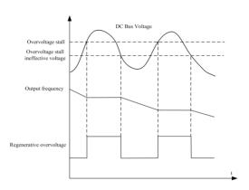
Figure 7-24 Overvoltage Stall Protection
