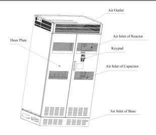
Figure 1-9 Description of Parts of EM500 Inverter (450kW)
