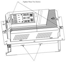
Flush Mounting Parts Installed Into the Plastic Shell Slots at Both Side:
