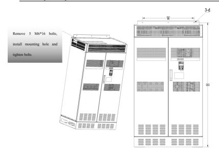
Figure 11-7 Installation of Upper Mounting Hole
