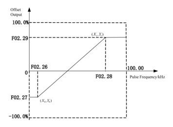
Figure 7-10 High-Speed Pulse Input Offset Curve
