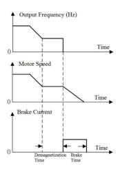
Figure 7-18 Start Process of DC Brake
