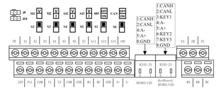
Figure 3-12 Control Circuit Terminal Block
