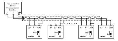
Figure 3-20 Wiring of Communication Interfaces of Multiple Inverters
