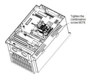
Figure 3 Installation of Profibus-DP expansion card
