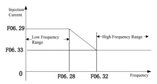
Figure 7-23 High Frequency Injection
