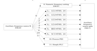
Figure 1-3 Auxiliary Frequency Source B Setting
