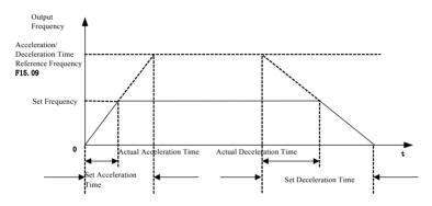
Figure 7-33 Acceleration/Deceleration Time
