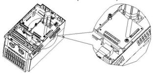
Figure 1 Installation of IO Expansion Card
