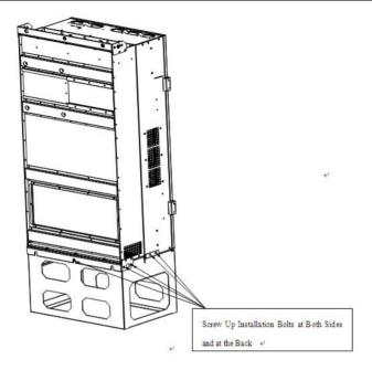
Figure 11-3 Base Installation
