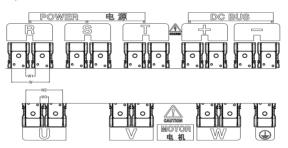
f) Main Circuit Terminal Block of Models 220 - 400 kW
